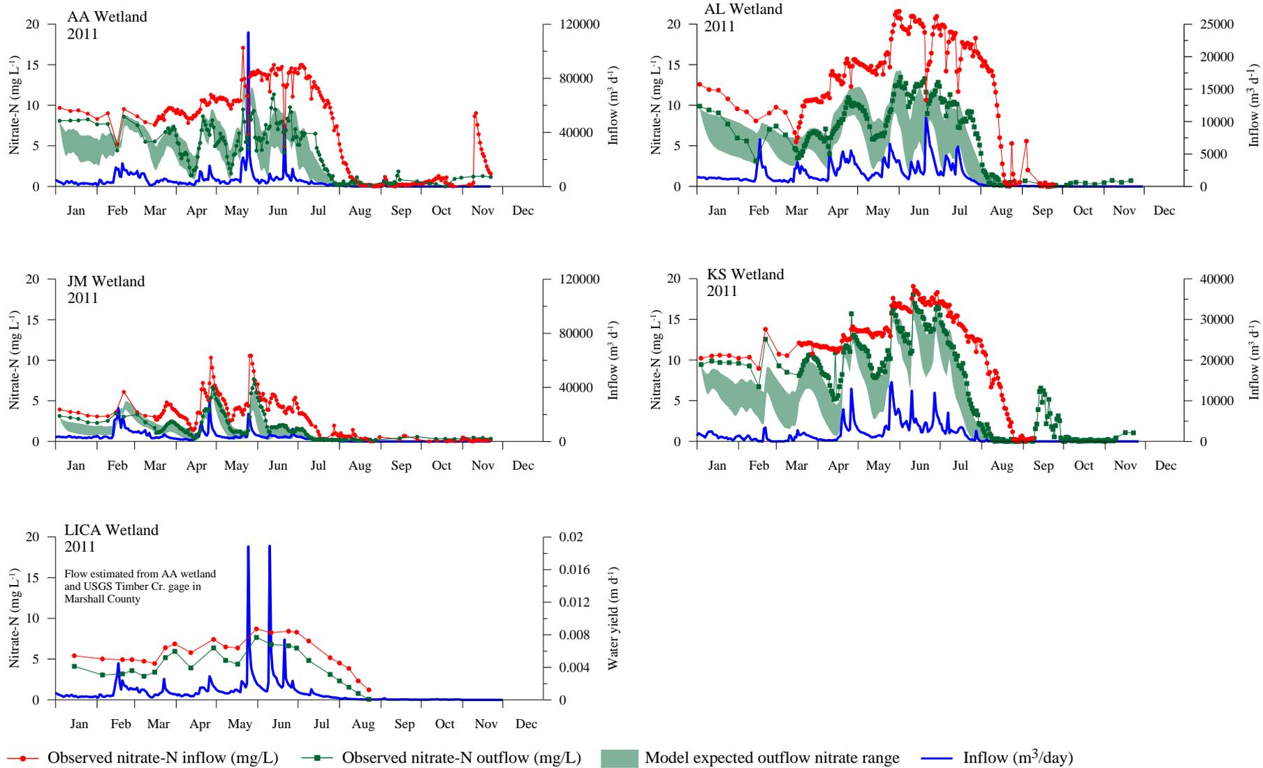
Figure 2. Measured and modeled nitrate concentrations and flows for wetlands monitored during 2011.
