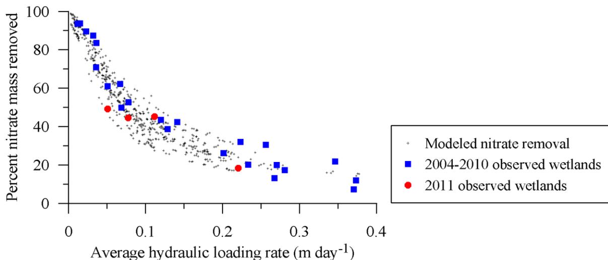
Figure 3. Modeled nitrate removal efficiencies for CREP wetlands based on 1980 to 2005 input conditions and measured nitrate removal efficiencies for CREP wetlands during 2004 to 2011.
